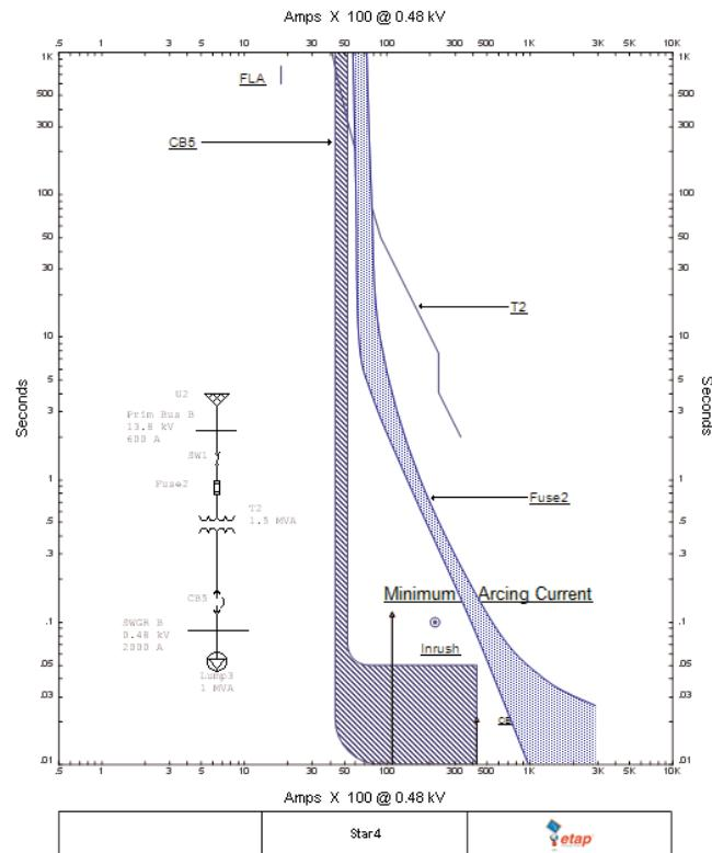
Figure 4: TCC showing Maintenance mode for CB5
