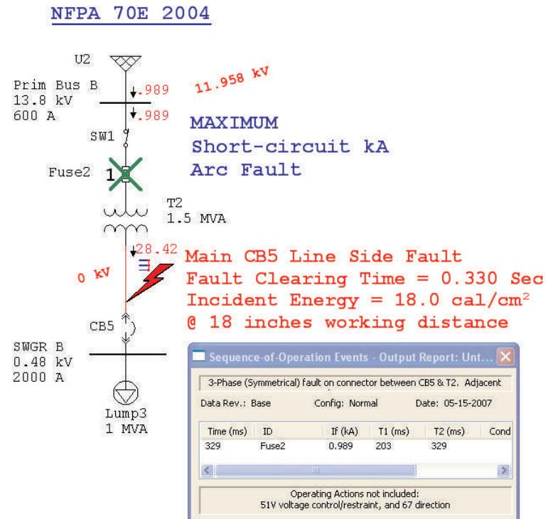
Figure 1: Arc Fault at line side of CB5 showing NFPA 70E results
