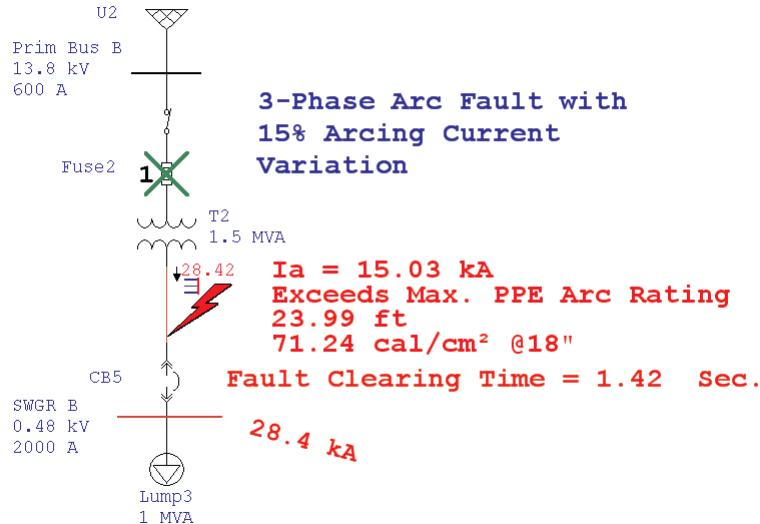
Figure 2: Arc Fault at Bus SWGR B showing IEEE 1584 results
